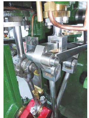
Fully Restore-d: engine cross head and valve motion
